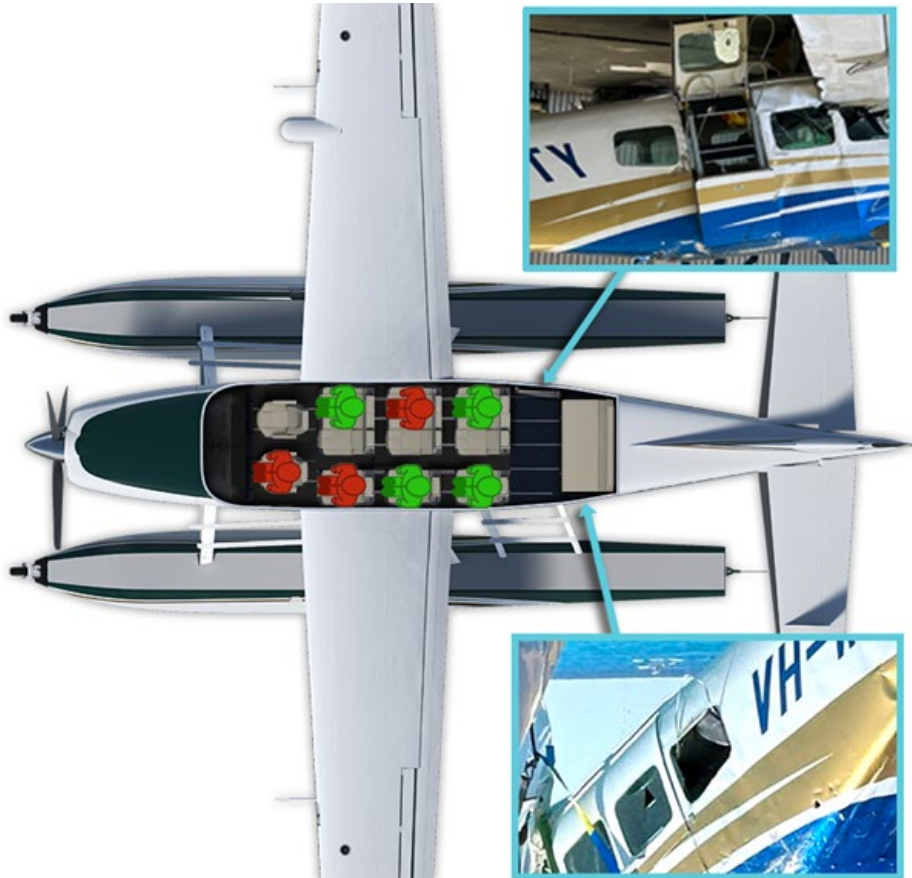
Figure 9: Cessna 208 seating plan showing the occupant location for those who survived (green) and those who sustained fatal injuries (red)
