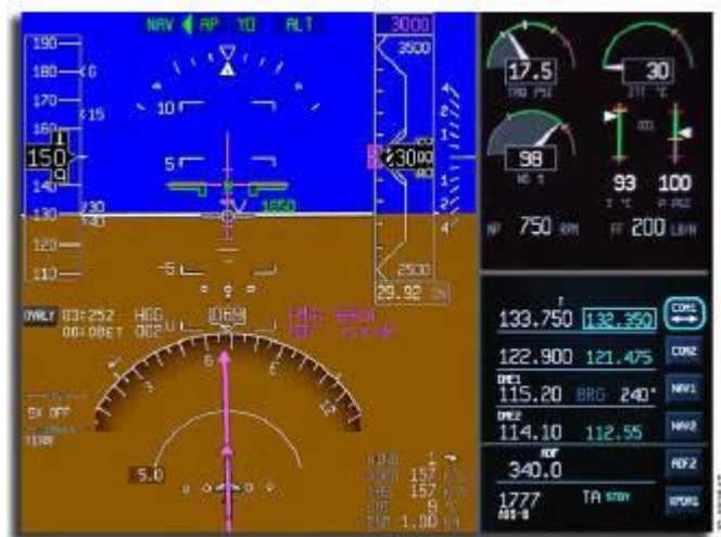
Figura 14: primary flight display da Honeywell Primus Apex Integrated Avionics System for the Pilatus PC-12 NG Pilot's Guide Rev. 20 del 6.1.2020 .
