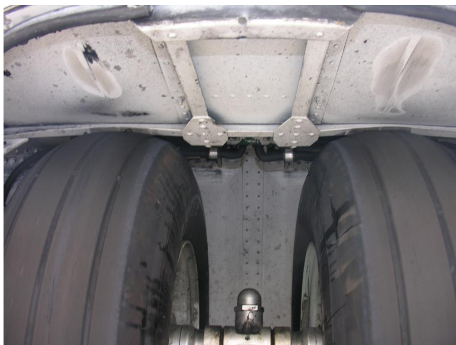
Photo 5: nose landing gear compartment.
