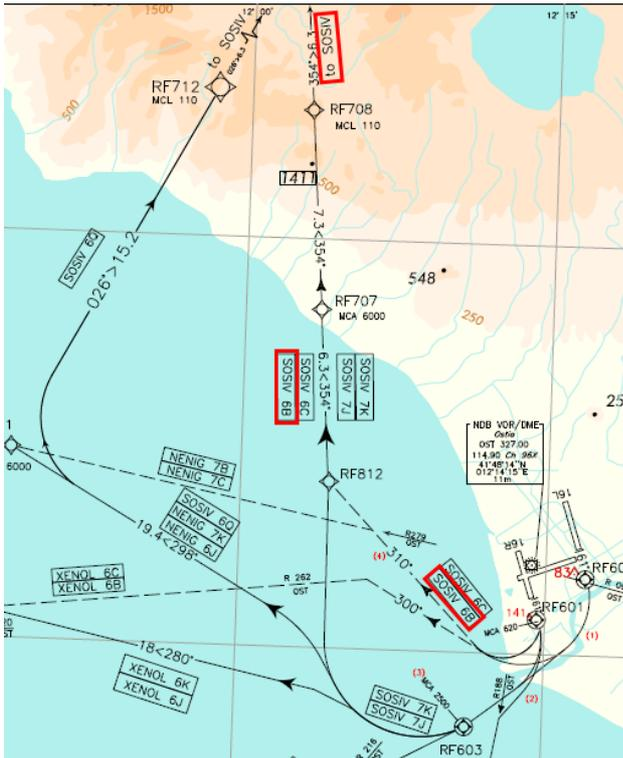
Figure 14: SID SOSIV 6B (source AIP Italy).
