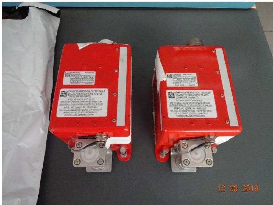
Photo 13: EAFR installed on board the LN-LND.
